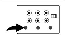
If the picture moves up and down or rolls, rotate to adjust the vertical hold.
